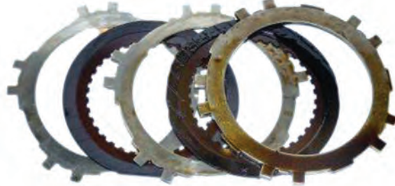
Automatic transmission clutch plates pre-cleanup. Varnish and glazing is heavy on some of the plates.
