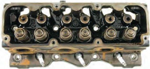
Cylinder head pre-cleanup. Note the sludge deposits on and around the valve springs and push rod openings.
